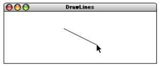
Because the original point and the mouse position appear to be joined by some elastic string, this technique is called rubber-banding. Although this program may seem quite powerful, it is also simple to implement. The entire program requires fewer than 20 lines of code.
